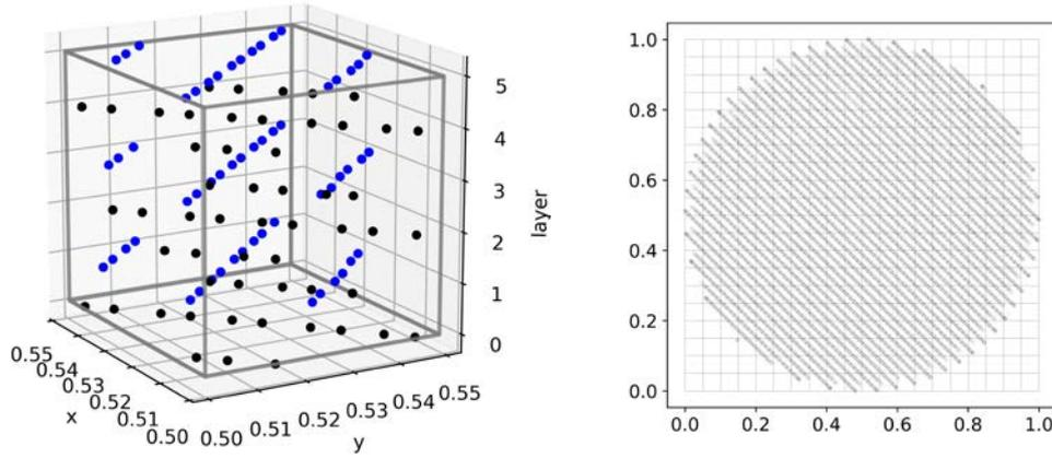
**Fig. 3** (a) schematic representation of a voxel and the correspondingly allocated melt pool data (b) schematic representation of 2D voxel grid and melt pool data of a single slice
