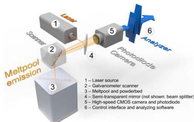
**Fig. 1** Main set up of QM Meltpool 3D system [1]
