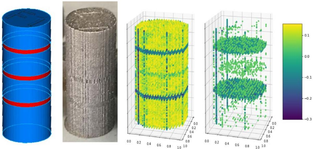
**Fig. 6** Validation specimen with build in error layers (model, real specimen and anomaly score plots)
